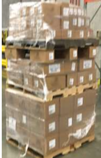
Improperly stacked pallets
