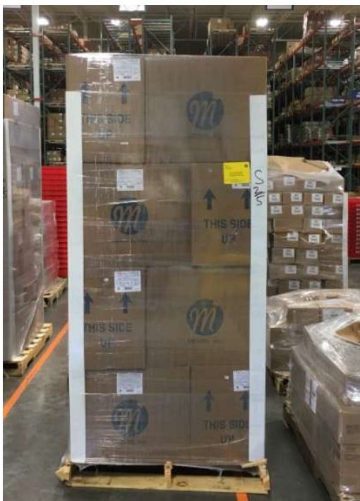
Improperly stacked pallet over 6'
